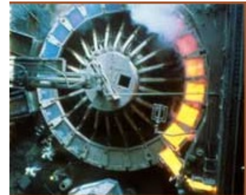
Picture 8. This huge wheel is used to cast the anodes. Molten copper is poured into a mould and the wheel is turned for the next mould. Meanwhile, the molten copper cools and solidifies into anodes over a metre tall.
